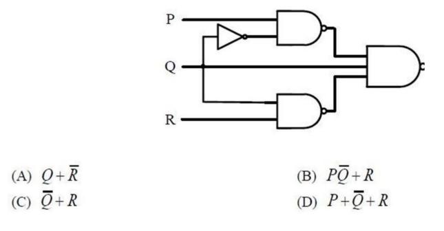
14. In the logic circuit shown in the figure, Y is given by
